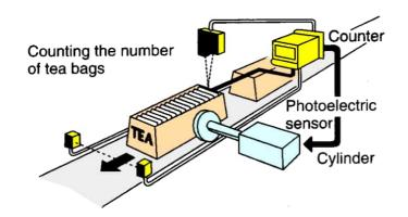
Machines that process thousands of items per second and objects that spend only a fraction of a second in front of a sensor require the PLC's quick response capability.
