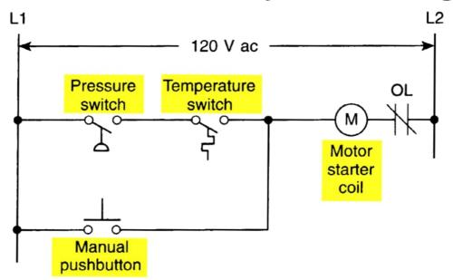
Motor starter coil is energized when both the pressure and temperature switches are closed or when the manual pushbutton is pressed
