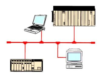
They can be networked to perform such functions as: supervisory control, data gathering, monitoring devices and process parameters, and downloading and uploading of programs.
