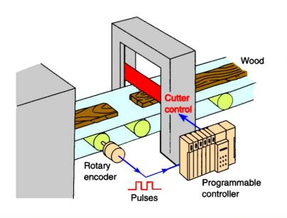
It is easier to create and change a program in a PLC than to wire and rewire a circuit. End-users can modify the program in the field.
